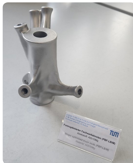
Figure 1. Truss node made of AlSi10Mg using PBF-LB/M
