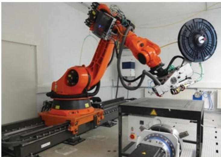
AFPT machine at LCC (Image courtesy: LCC)
