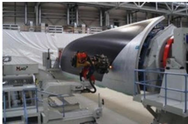
Typical fiber placement (Image courtesy: Premium Aerotec GmbH)
